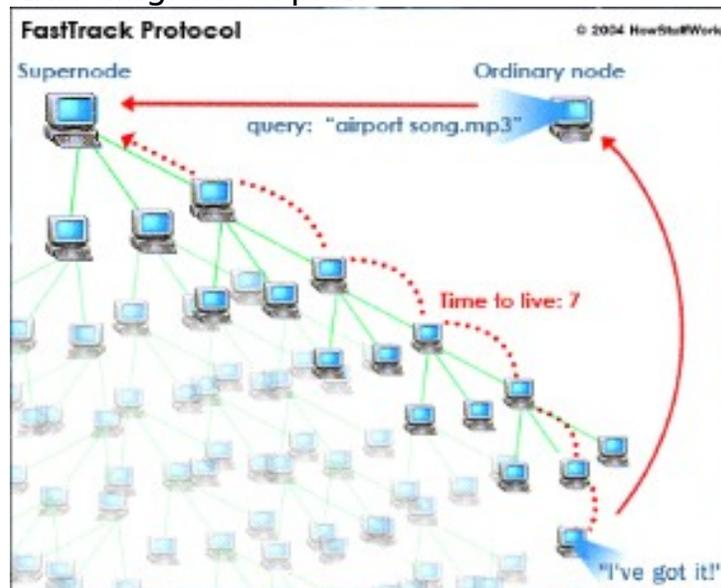
*Structure of the FastTrack peer-to-peer file sharing network used by the P2P program Kazaa.*
